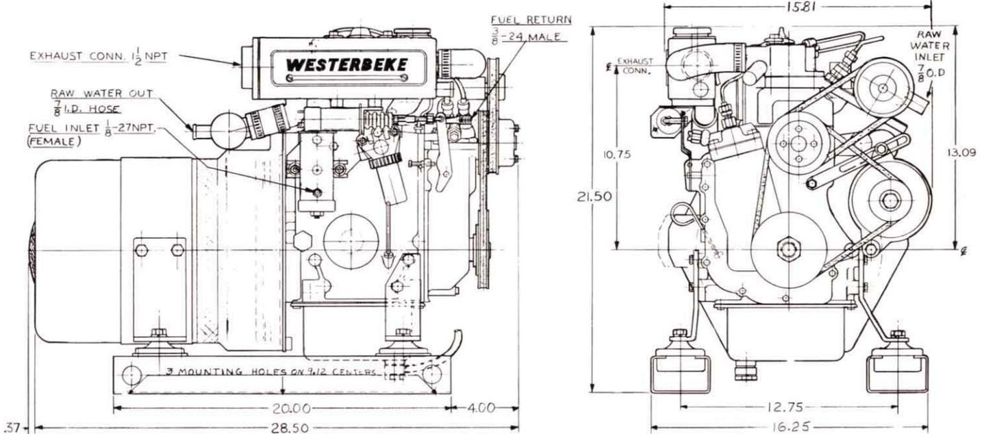
**DESIGN:** Four pole revolving armature, inherently regulated, self limiting, rectifier excited, A.C. slip rings, single bearing design.
